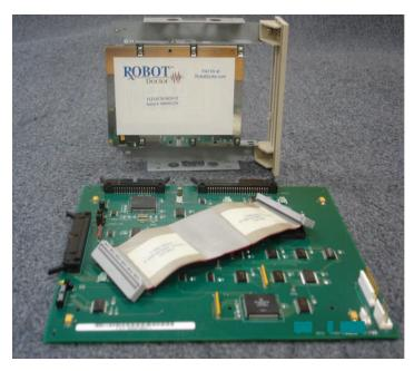
If you've ever suffered production down time from a failed Multibus hard drive board in your Adept MC controller, you'll appreciate our Solid State Flash Drive replacements. These Flash Drives contain no moving parts so there is nothing to wear out. Flash drives are available in 10 or 20Mb storage sizes depending on V<sup>+</sup> version. They are also available for IC, CC, MC and OC Adept controller models.
